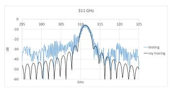
Fig. 7. Spectrometer room temperature test results and responses calculated through ray tracing around 190 GHz, 241 GHz, and 311 GHz, respectively.
