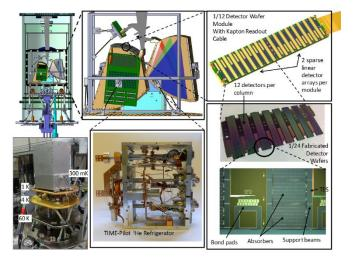
Fig. 1. TIME-Pilot instrument overview.
