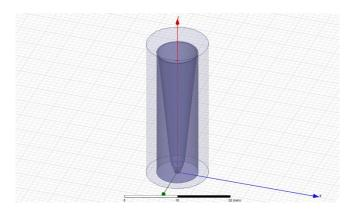
Fig. 3. HFSS model of the three-section MFA horn.
