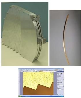
Fig. 6. Two-channel grating spectrometer stack with input and output feeds connected. The 190 facets on the grating were wire-cut. A close-up view of the grating facets is also shown.
