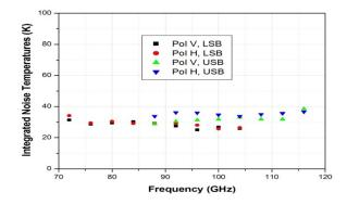
Fig.5: Integrated noise temperatures of the 71-116GHz RF module (including the OMT).
