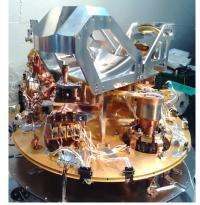
Fig.6 : Integration of the 3mmupgraded module into the EMIR receiver.
