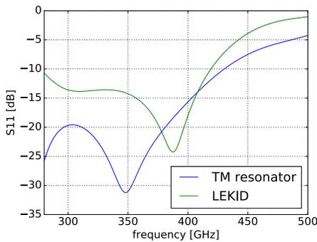
Fig. 2. CST<sup>TM</sup> microwave studio simulation results of the input reflection ( $S_{11}$ ) seen from the waveguide for the high frequency signal input for the transmission line resonator design (TM) and the lumped element design.
