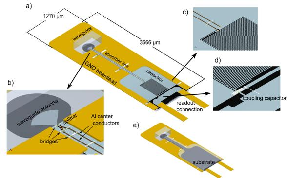
Fig. 3. CAD rendering of the lumped element resonator design. a) Overview b) Waveguide probe section with splitter. c) Transition from absorber line to capacitor. d) Coupling to the readout line.
