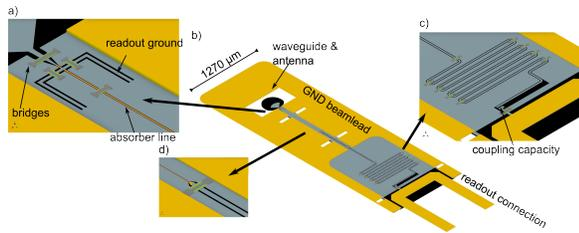
Fig. 1. CAD rendering of the transmission line resonator design. a) Waveguide antenna and choke. b) Overview of the chip. Dimensions are 1.2 by 3.6 mm. c) Meandered resonator line and coupling to the readout. d) Transition from aluminum absorber to the niobium resonator line.
