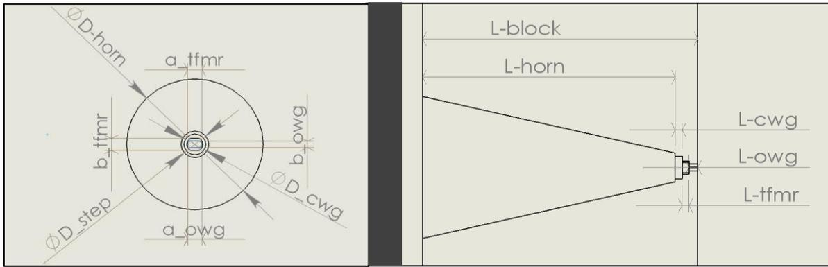
Fig. 1. Critical dimensions of the design model of the waveguide circuitry of the horn-transformer module as seen looking down the aperture (a) and a cut across the profile (b). Dimensions of these features are listed in Table I. The horn is located in the middle of a 20 mm square block of 145 copper (ultra-high purity) copper alloy. A set of four guide pins spaced on the flange outside the frame of this model image ensured precise alignment to the mixer backend.
