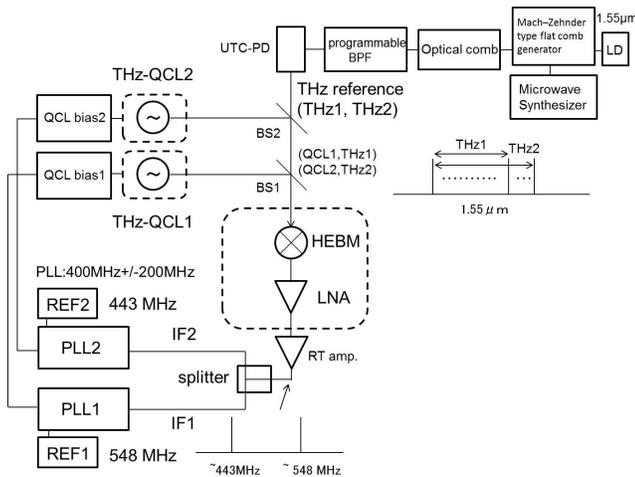
Fig. 1. A system block diagram of simultaneous phase-locking of two THz-QCLs using an HEBM and an optical comb generator followed by a UTC-PD.
