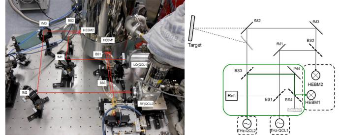
Fig. 4. System block diagram of a THz radar system (above), a photograph of an experimental setup (bottom left), and modified optics (bottom right).
