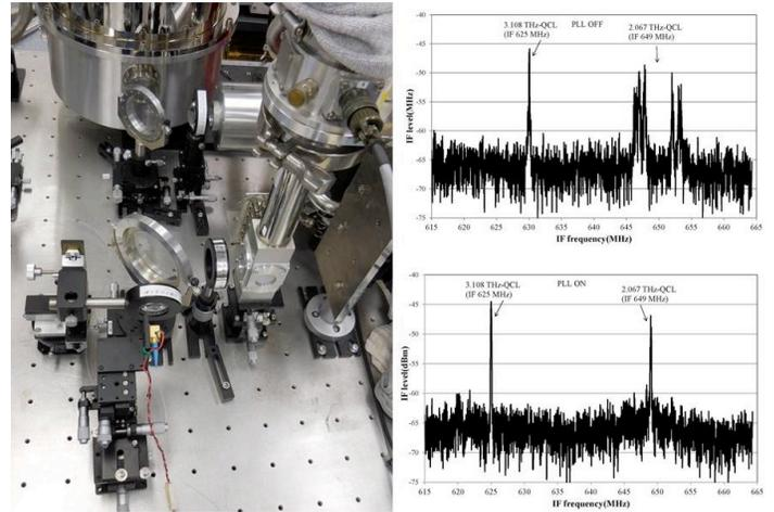
Fig. 2. A photograph of setup for the simultaneous phase-locking of two THz-QCLs (left). Each THz-QCL was cooled by different cooler, 45 K mechanical cooler and a LHe flow-type cryostat. THz reference was generated by a comb generator followed by a UTC-PD. Mylar beam splitters were used for LO injection to an HEB mixer. The detected spectrum show beat signals of PLL OFF(upper right)/ON(lower right) for 2 THz and 3 THz-QCLs.
