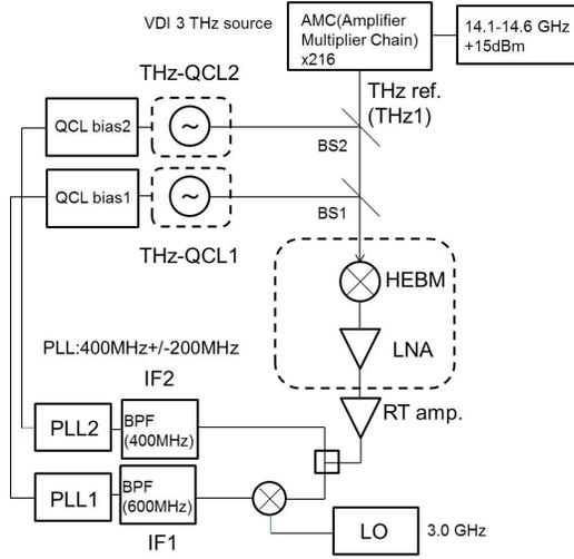
Fig. 3. Phase-locking system of two THz-QCLs using an AMC as a THz reference. In this case, we have a single THz reference signal. Therefore, the lasing frequency of two THz-QCLs should be within an IF bandwidth of an HEBM. Although, the gain IF bandwidth of the HEBM is around 3 GHz, the beat signal can be detected even at  $\sim 14$  GHz if we use an appropriate LNA.
