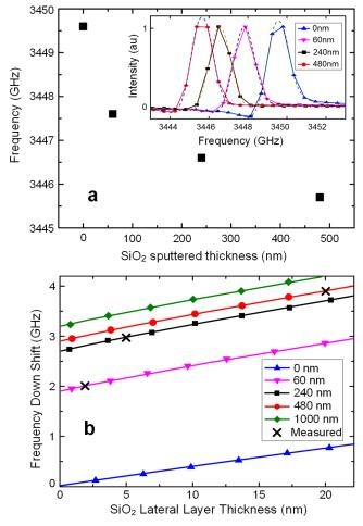
Fig. 2 a) The measured frequencies of the 3.5THz QCL before and after of the SiO2 sputtering in thicknesses of 60, 240 and 480nm. Inset shows the raw FTS spectrums (solid lines) together with the fitted curves (dashed lines). b) The simulated dependence of the frequency downshift on the lateral layer thickness, in five surface layer thicknesses of 0, 60, 240, 480 and 1000nm. The crosses show the experimental data points.
