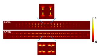
Fig. 2 Top view of the normalized magnitude of the extending electric field to the free space of two QCLs at 3.5 THz and 4.7 THz used for our experiments, showing different field distributions.
