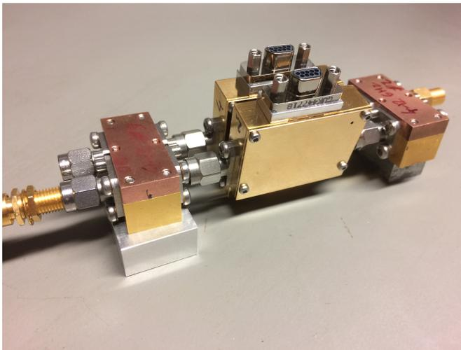
Fig. 2 Balanced amplifier based on the 4-12 GHz hybrids.
