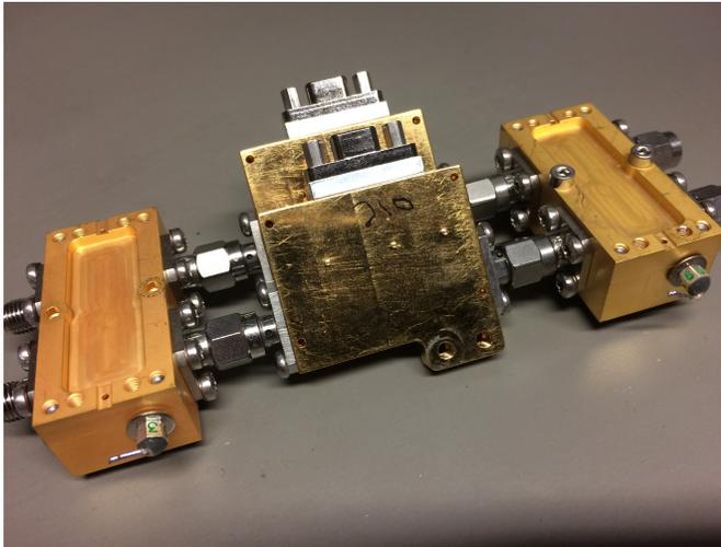
Fig. 1 Balanced amplifier assembly based on 4-8 GHz hybrids
