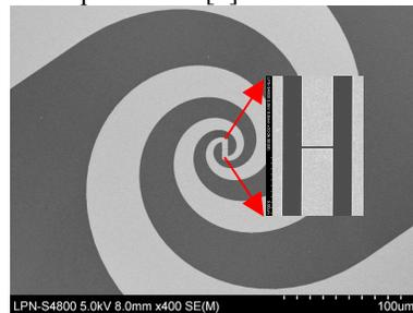
Fig. 1. SEM image of a log-spiral antenna integrated NbN HEB mixer on silicon. The light gray area is the gold antenna structure, while the dark area is the Si substrate. The close-up picture shows the structure of micro-bridge.
