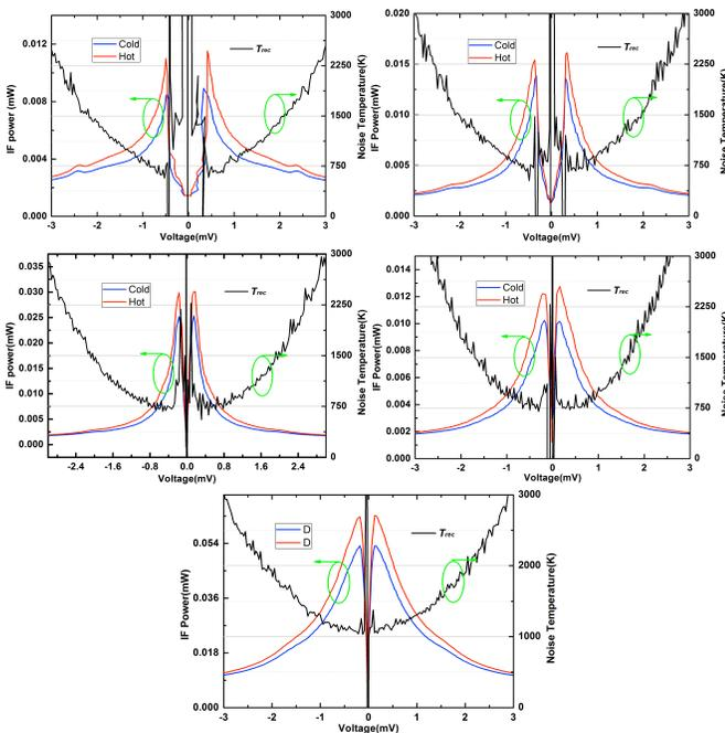
Fig. 3. Measured receiver IF output power (left axis) for the hot-and cold-load at an optimal LO power and the corresponding DSB receiver noise temperature (right axis) at 0.2 THz, 0.5 THz, 0.6 THz, 0.85 THz and 1.34 THz, shown as a function of the mixer dc-bias voltage.
