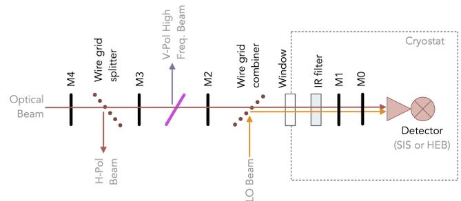
Fig. 4. Diagram showing the main optics components. 4G-4 uses a diplexer instead of a wire grid as combiner. The beam optics comprises two Gaussian telescopes: M4-M3 (at the Optics Plate) and M2 (Optics Plate) with M1 (Cold Tower).
