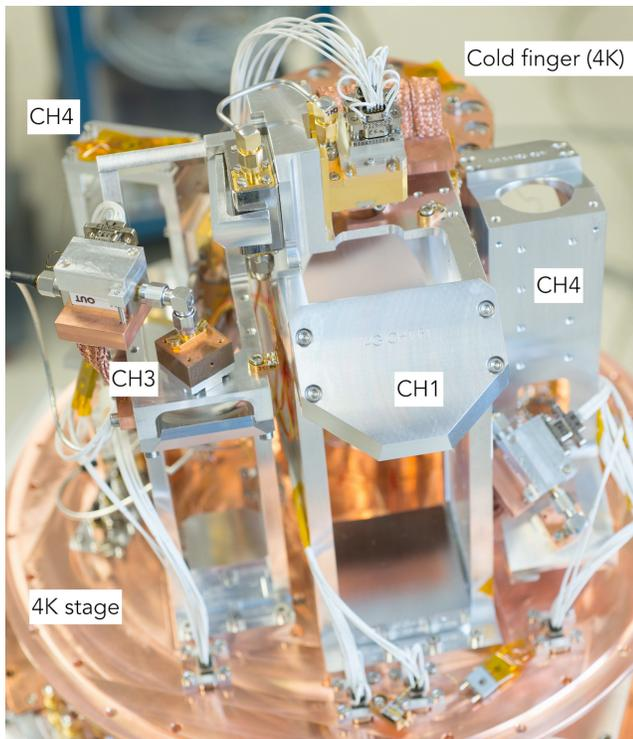
Fig. 3. Each *cold tower* mounts a paraboloidal (M0), a flat and an ellipsoidal mirror (M1), along with the corresponding mixer and cold LNA amplifier.
