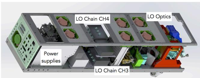
Fig. 7. The lower LO unit (serving 4G3 and 4G-4) is a very compact unit that includes its power supplies, the LO chains and the LO fore-optics.
