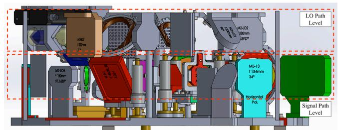
Fig. 5. Side view of the optics plate. Red dashed lines frame the two planes. Some non-critical elements have been omitted in the figure for better visualization.
