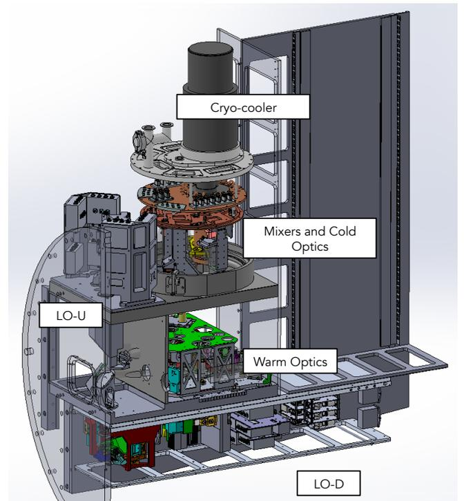
Fig. 2. 4GREAT subcomponents mounted on the GREAT SI structure: The cryostat (mixers, cooler and cold optics), the lower local oscillator unit (LO-D), the upper local oscillator unit (LO-U) and the warm optics are shown.
