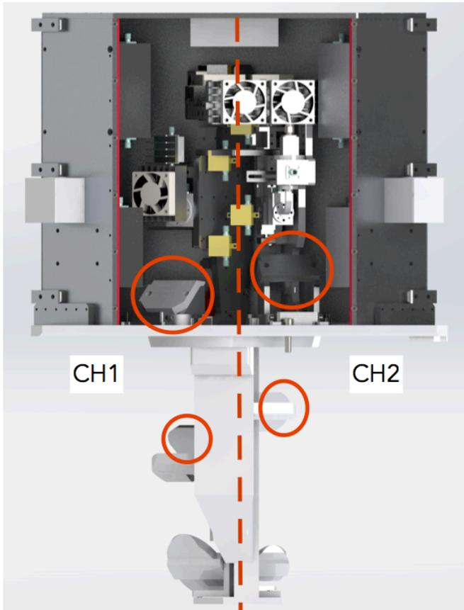
Fig. 6. The upper LO unit (serving 4G-1 and 4G-2). The LO chains and optics components are visible in the image. The two active mirrors for each LO are encircled. The dashed line indicates marks the optical and electrical separation between the two channels.
