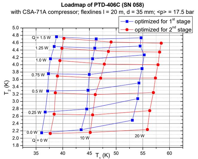
Fig. 8. Thermal load map for the Pulse Tube cooler used by 4GREAT. The operation temperatures are 3K (second stage) and 55K (first stage).
