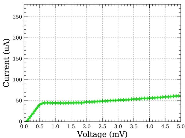
Fig. 9. Pumped I-V curves of the channels 4G-1, 4G-2 and 4G-4 mixers at 3.5 K. Curves for channels 1 and 2 were obtained with magnetic field applied.
