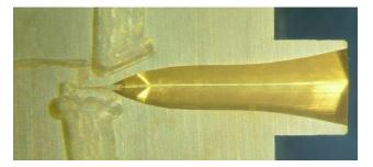
Fig. 2 1.2THz Sub-harmonic mixer split-block including spline diagonal horn antenna (design by GMD, machined by RPG Radiometer Physics GmbH)
