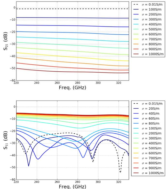
Fig. 3 Insertion loss (top) and return loss (bottom) of the full device as modelled by ANSYS HFSS for varying levels of substrate conductivity. It is assumed that illumination only changes the conductivity over a 200 $\mu\text{m}$  long section of the silicon probe chip.
