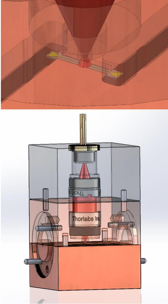
Fig. 2 (Top) View of probe chip as assembled in the waveguide block. Light passes through a small hole in the upper cavity onto the chip. (Bottom) Completed assembly of waveguide split-block and laser diode block. Shown in red is the beam of the 808nm laser diode as collimated and focused by the two-lens system.
