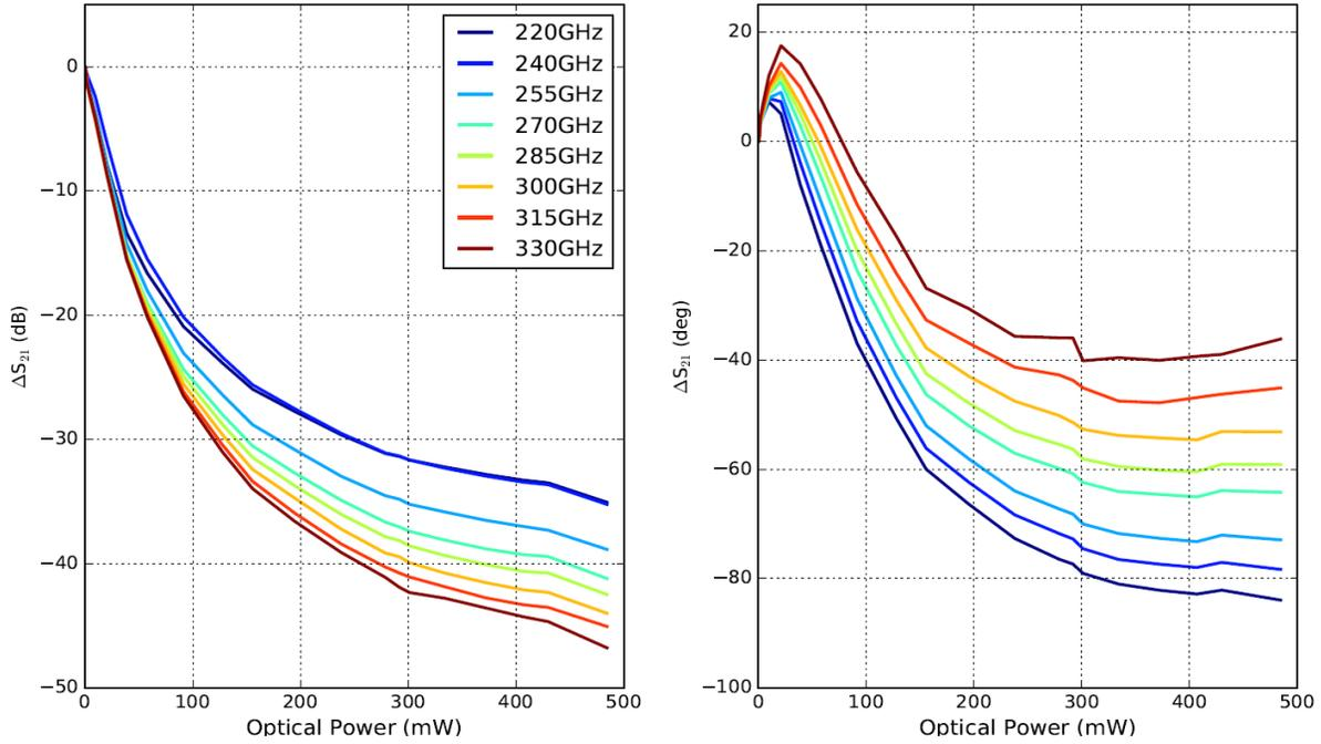
Fig. 6 Measurements of device insertion loss (left) and phase shift (right) versus incident optical power at 808nm for several frequencies across the WR3.4 band. HFSS modelling predicts a linear relationship between conductivity and insertion loss, which is seen for low incident power.
