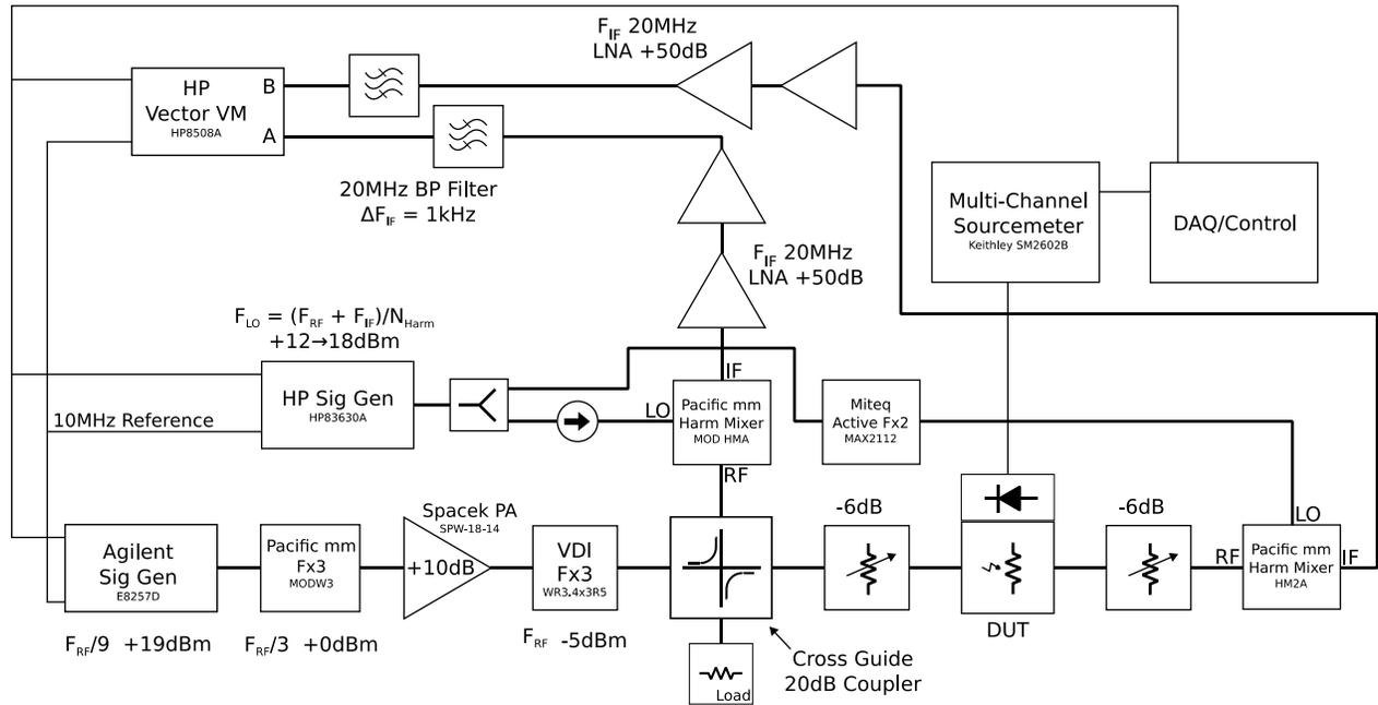
Fig. 4 Schematic of transmission measurement scheme. A coupled portion of the RF signal and the remainder after passing through the DUT are sent through a down-converting and amplification chain to an HP8508A Vector Voltmeter for measurement of the relative amplitude and phase of the transmitted signal.
