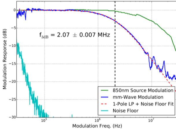
Fig. 7 Measurement of the modulation bandwidth of the device using a 20MHz 5mW IR LED source. A 3dB bandwidth of more than 2MHz is measured corresponding to a  $\sim 77$ ns carrier lifetime.
