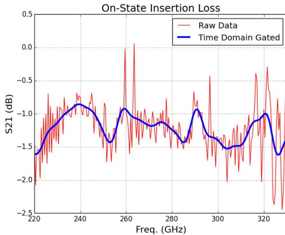
Fig. 5 Measurement of the insertion loss of the device in the no illumination or on-state. Time domain gating was applied to systematically smooth the data.
