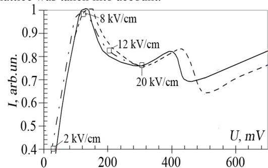
Fig. 2. Experimental line (solid line), inverse (dotted line) and calculated (dash-dotted) volt-ampere characteristics for 6-period SL. The abscissa represents the total voltage applied to the diode. The ratio of the field strength in the superlattice and the external supply voltage was determined by taking into account the resistance of the contacts. The figure shows the applied field to the diode.
