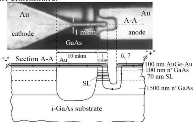
Fig. 1. Design of the planar diode heterostructure. Label "SL" and hatching marked the working area of the diode. Diode working area means the place of high current density flow. This area determines the external parameters of the diode. The heterostructure parts with low current density do not play a fundamental role in the operation of the diode. They are not hatched and are not marked with the label "SL".
