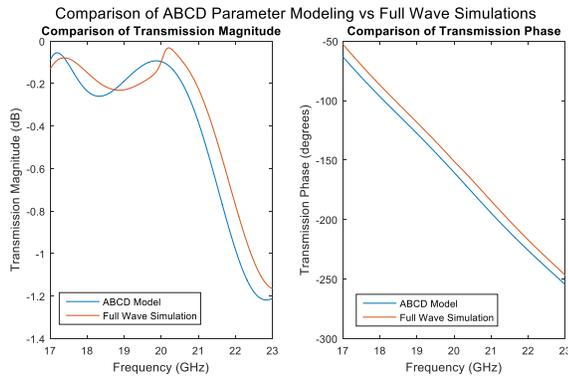
Fig. 3. Comparison of TL theory model vs. full wave simulation
