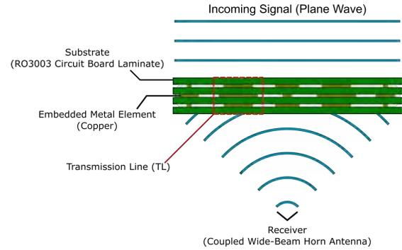
Fig. 1. Schematic diagram of metamaterial lens, not to scale
