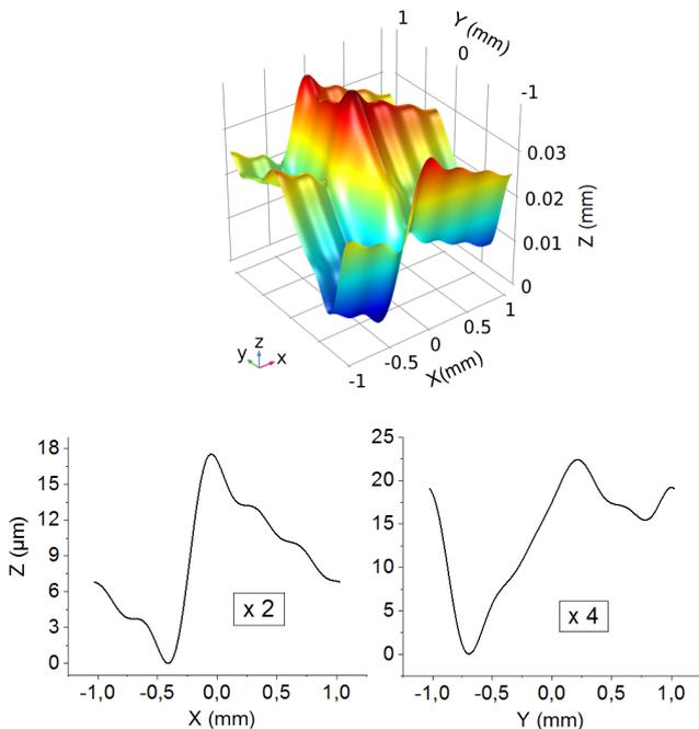
Fig. 1. 3D plot of the designed surface profile (top). At the bottom, orthogonal cross sections are plotted, each multiplexing the beam to 2 (left) or 4 (right).
