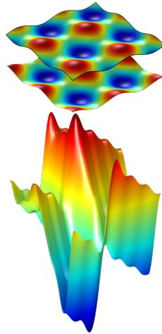
Fig. 1. Applied sine variations with 1 mm of period and 1  $\mu\text{m}$  of amplitude on top of the grating surface profile.
