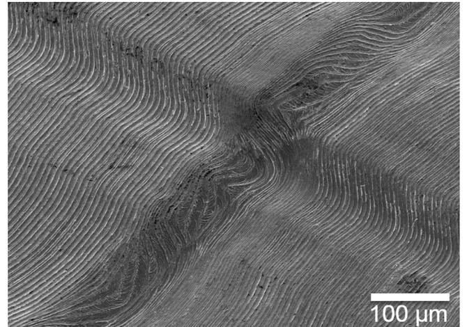
Fig. 2. An SEM photo of the machined 4.7 THz grating reported in [2].
