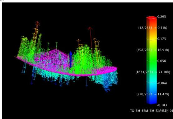
Fig.6. Distribution of residual error for prototype panel by photogrammetry
