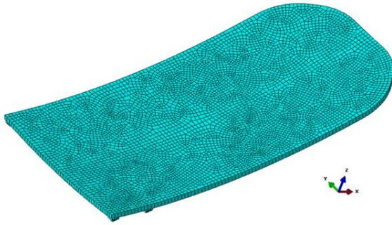
Fig. 1. Finite element model of primary reflector for MSX.
