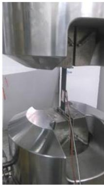
(a) Tensile test for M55J
