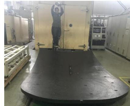
Fig.5. Surface measurement of prototype panel by photogrammetry
