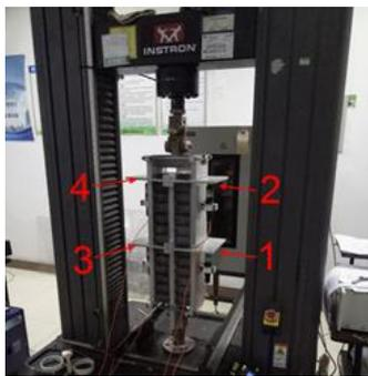
(c) Shear test for CFRP tube array
