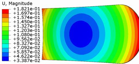
(a) Panel with CFRP tube array core
