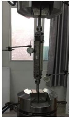
(b) Shear test for Al honeycomb
