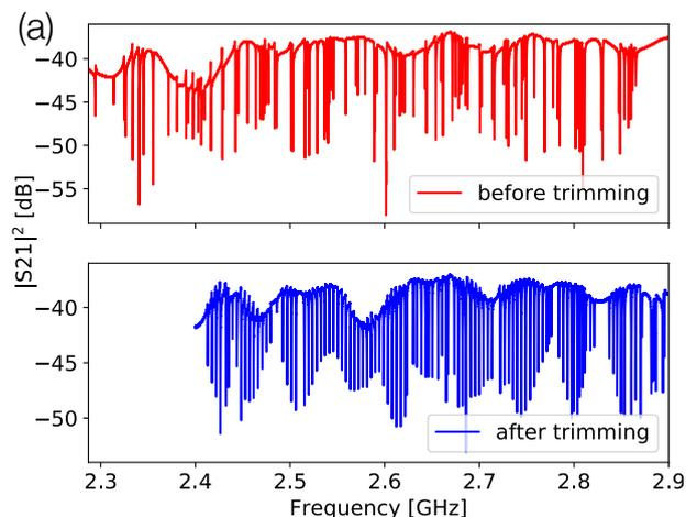
Fig. 1. Feedline transmission of the KID array before (up) and after adaptation of the individual pixels. The necessary readout bandwidth is reduced from 562 MHz to 490 MHz, whereas the frequency scatter with respect to the design value is reduced from  $\sim 2\%$  to  $\sim 0.02\%$ .
