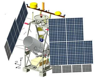
*GUSTO* ballooncraft and payload include a 0.9 m telescope, cryogenic THz receivers, and a gyro stabilized pointing system to provide an unparalleled galactic-extragalactic survey capability.
