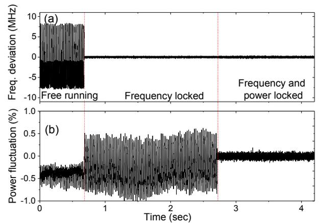
Fig. 1: (a) Frequency and (b) output power stability for the three cases: free running, frequency locked, frequency and power locked.
