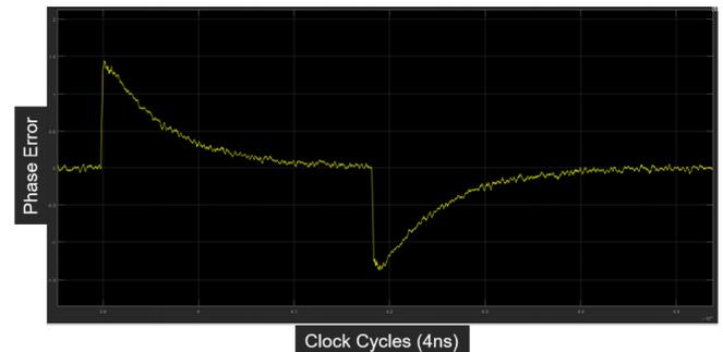
Fig. 6. Noisy simulation showing two simulated resonance shifts both finding the resonance on millisecond timescales.
