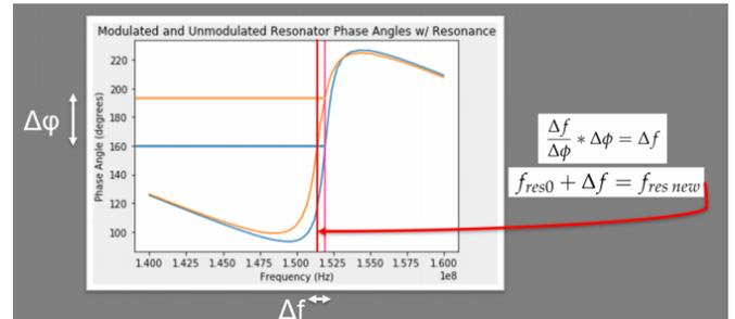
Fig. 3. A graphical representation of the tone tracking algorithm.
