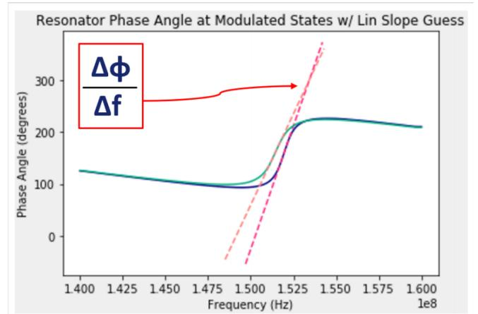
Fig. 2. A plot highlighting the linear regime in the phase/frequency relationship of a resonator in both the rest state and a modulated state. Previous applications of KIDs have confirmed that resonant frequency will not stray from this linear portion. While modulation of the KID causes changes in slope, the tone tracking system is designed in a way where these differences can be ignored.
