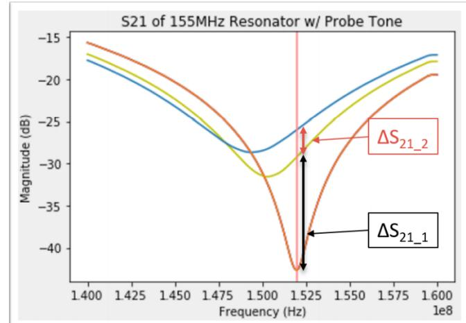
Fig. 1. An exaggerated example depicting the diminishing returns of incident power on a KID. Increasing power returns smaller and smaller changes in amplitude until the difference between two modulated states is dominated by amplifier noise. As of now, the only correction possible is a time-intensive mid-flight VNA sweep.
