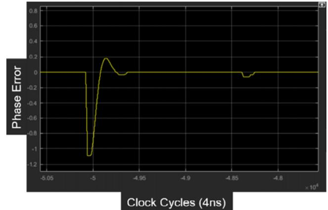
Fig. 5. Noiseless simulation results of tone-tracking algorithm measuring the difference between the real-time phase and resonant phase. Zero means the tone is tracked. The first spike represents a large phase shift and a damped oscillation is visible. The second bump is a much smaller and more realistic phase shift.
