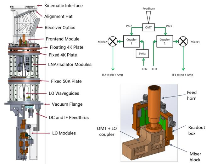
Fig. 7. (left) CAD rendering of populated wSMA receiver cartridge, with LO module installed. (upper right) Schematic of the wSMA receiver frontend, and (lower right) CAD rendering of a wSMA receiver front-end module.
