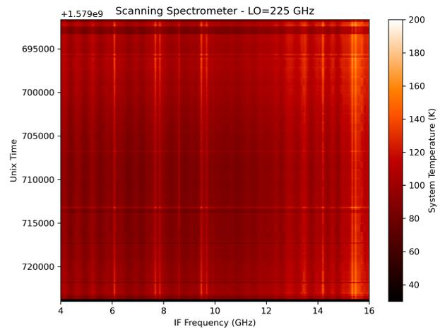
Fig. 9. Scanning spectrometer DSB  $T_{\text{sys}}$  data for one frequency recorded during a test observation. Vertical lines in the data correspond to stratospheric ozone lines in one of the two sidebands. Sharp horizontal lines correspond to rapid changes in the telescope pointing to switch to flux calibration and pointing targets, while slow variations track changes in atmospheric conditions and observation target elevation.
