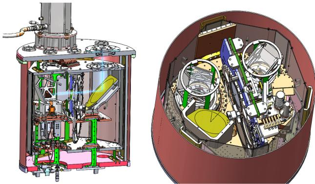
Fig. 4. Cut-away CAD renderings of the wSMA cryostat, showing the cryostat structure and the optical layout (optical path highlighted in blue on the left image). Renderings courtesy of HPD Inc.
