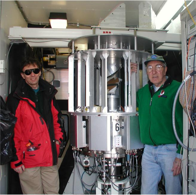
Fig. 1. SMA receiver and receiver optics cage in an SMA antenna, circa 2005. (with John Barrett and SMA Director Raymond Blundell). The SMA beam waveguide mirrors M6 and M5 are visible at the top of the image, with the optics cage containing the moving wire grid and mirror combiners below the cross-beam. The cryostat is below the optics cage, with the receiver electronics “cheeks” mounted around it.
