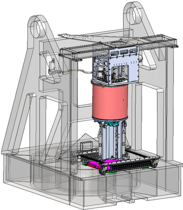
Fig. 2. wSMA Receiver cryostat (vacuum shell in pink), support structure and alignment structure in the SMA receiver cabin (existing structures are transparent). Rendering courtesy of HPD Inc.
