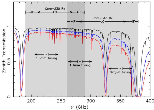
Fig. 3. wSMA receiver bands sky frequency coverage, overlaid on Maunakea sky transmission for the best 50%, 25% and 10% weather.
