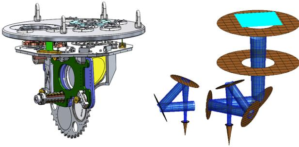
Fig. 6. (left) CAD rendering of the cryostat fold mirror and selector wheel supported from the upper vacuum plate and upper radiation shield plate of the cryostat. Rendering courtesy of HPD Inc. (right) GRASP model of the cryostat and receiver optics showing the Gaussian beam envelopes as the beams from each receiver feed pass through the receiver optics, selector wheel, fold mirror, and IR filter and vacuum window apertures.
