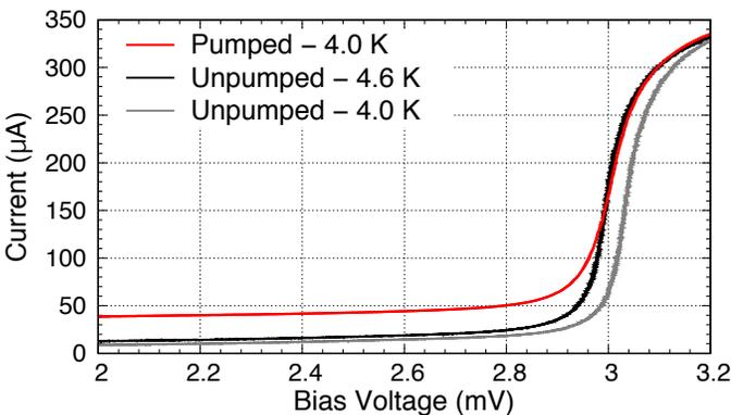
Fig. 2. Plot illustrating how we infer the effective temperature of the tunnel junction by matching the gap voltage of pumped and unpumped IV curves at different block temperature. The temperature shown in the legend indicates the mixer block temperature when the IV curve was taken.
