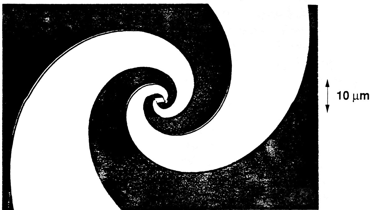
Figure 1. Photograph of the antenna-coupled microbolometer
