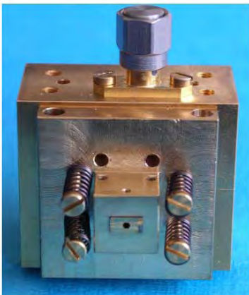
Figure 1: 600 GHz split-block mixer
