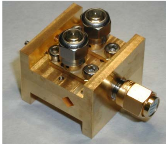
Fig.5. Photograph of the final integrated mixer/multiplier assembled block.
