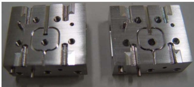
Fig. 12 Split-block view (Top) and assembled Band 4 OMT block (Bottom)
