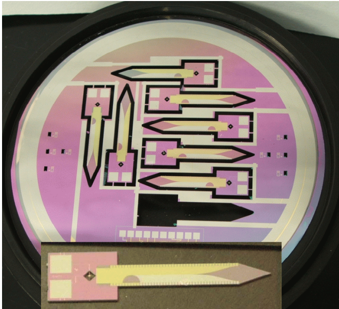
Fig. 4 Prototype 97-GHz C_0 over detector chips fabricated on a 2" wafer and (inset) an enlarged view of an individual chip. The chip is about 17 mm long.
