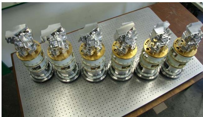
Fig 2, Photograph of six ALMA band 9 cartridges of a series of eight pre-prototypes, two cartridges have already been delivered to the ALMA project.
