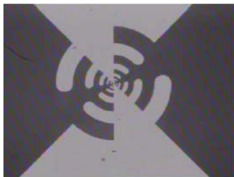
Figure 2. LPA2 with 1 \mu\text{m} gap used in later THz measurements.
