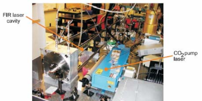
Figure 11. The \text{CO}_2 -laser pumped THz gas laser
