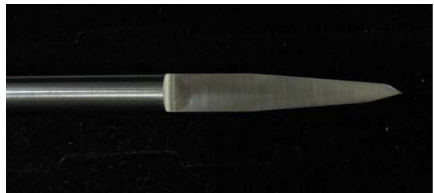
Fig. 5 The tool used for machining the three-section, 230 GHz horn. The cutting edge along the top of the tool has the required shape of the horn profile
