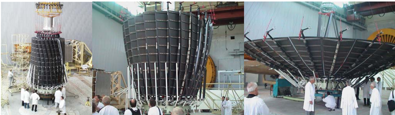
Fig. 2 Different stages of the "RadioAstron" 10m antenna deployment at Lavochkin Association (Moscow, Russia).
