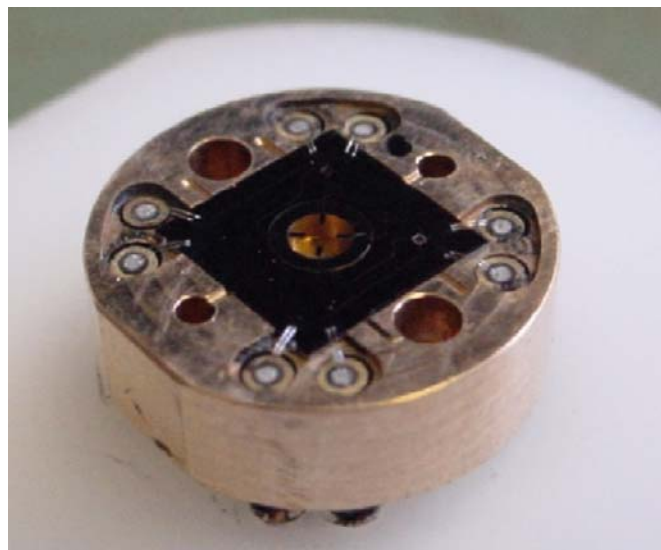
Fig. 12 150-GHz prototype detector mounted on a chip holder. Electrical connections are made from the chip to copper-clad aluminium pins which are fed through to the bottom of the holder where they are soldered into a PCB. There is a quarter-wave recess in the block under the nitride membrane.
