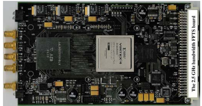
Fig. 9 Currently in development: The 2.5 GHz bandwidth FFTS. The board makes use of a first sample of E2V's 5 GS/s 8-bit ADC.
