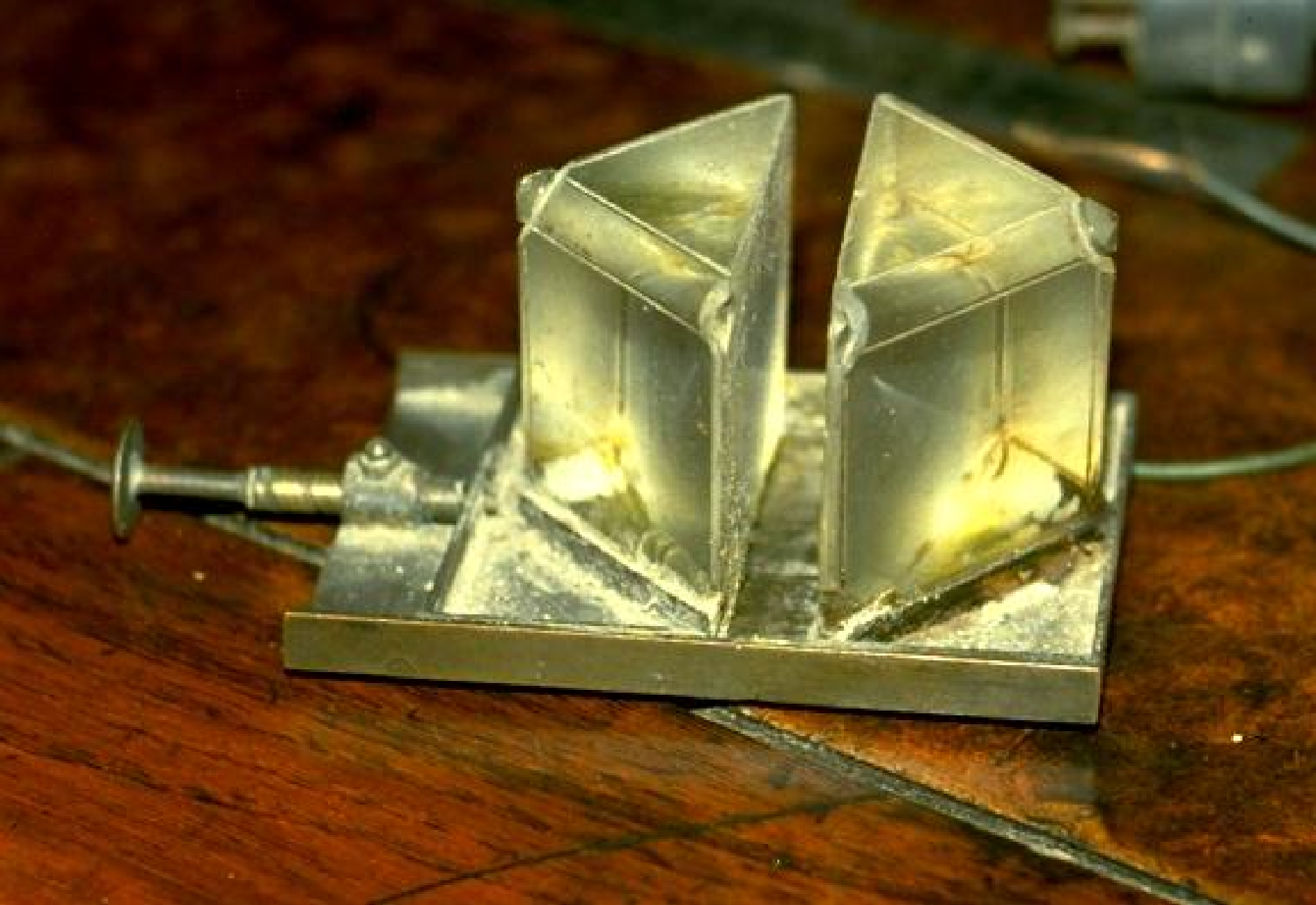
J.C. Bose dual prism microwave attenuator with adjustable air gap. Calcutta 1896
