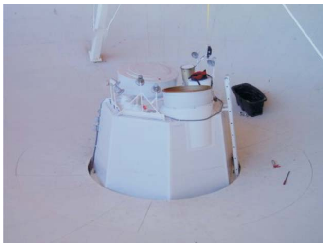
Figure 2. First S-Band feed horn installed in an EVLA antenna.
