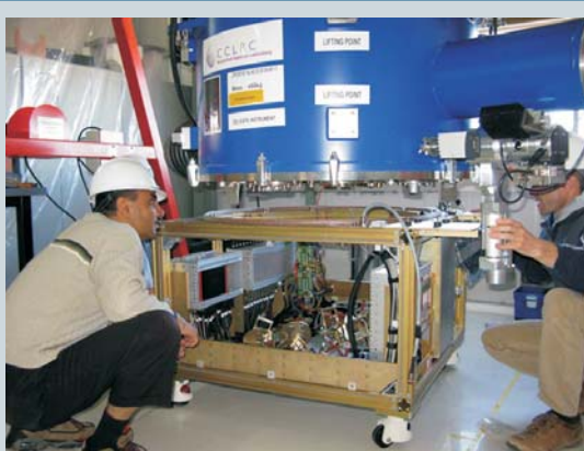
Figure 4. The first ALMA Front End undergoes provisional acceptance at the OSF in May. The sensitive detectors are in the large blue dewar, which keeps them temperature stable at near absolute zero.
