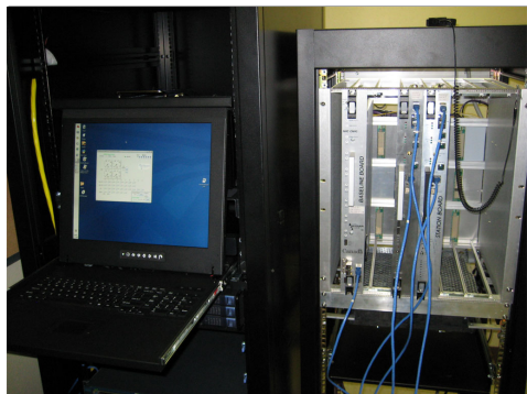
Figure 1: The Prototype Correlator for the EVLA in the old correlator room at the VLA site. The right-hand half-rack houses the correlator boards: two Station Boards to filter receive and sub-divide the data from two antennas, and one Baseline Board to perform the cross-correlations. The left-hand rack houses several associated general-purpose computers which control the correlator and process and archive the correlator output data. Two more Station Boards will be added over the next few weeks, giving four antenna and full closure capability.
