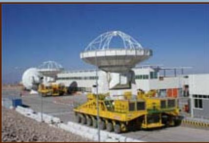
Figure 3: Vertex antennas No. 4 and No. 2 were moved to new foundations at the Operations Support Facility as testing continued. Photo: Luis Roa.
