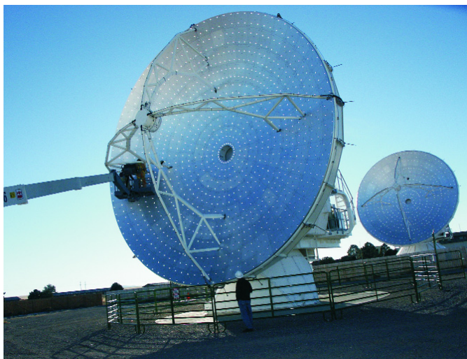
Vertex antenna (foreground) being fitted with photogrammetry targets at the ATF. Mitsubishi antenna shown in background. (Photograph by Fred Schwab)
