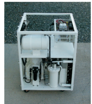
Figure 4. St. Croix cryogenic compressor after reconditioning.
