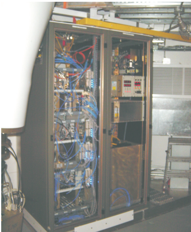
Figure 1. The EVLA electronics racks, located in the antenna vertex room. The large white object on the left is the bottom end of the new L-band horn.
