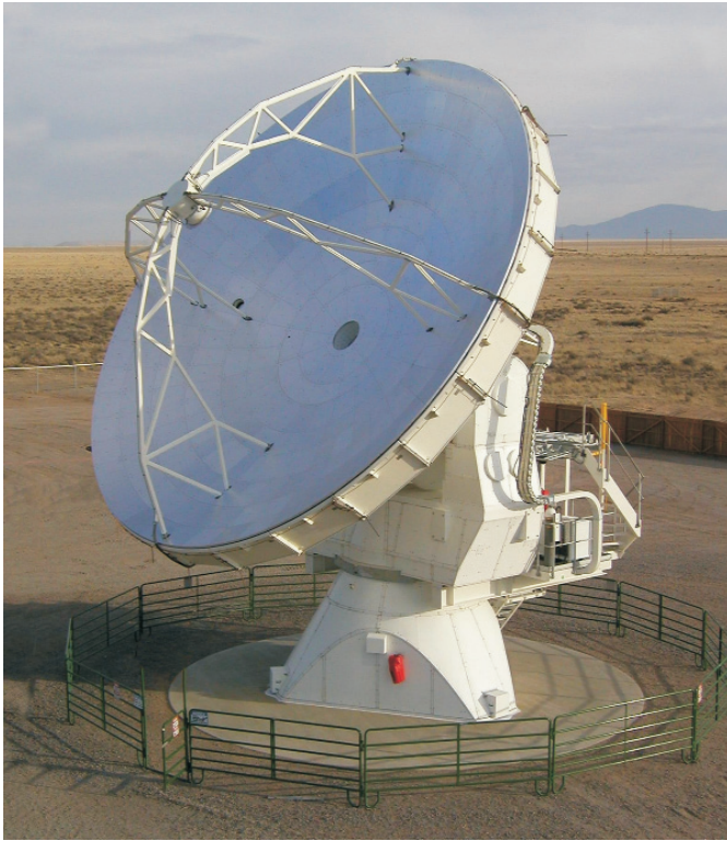
Figure 1. The VertexRSI antenna, a prototype for the ALMA production antennas, has undergone extensive testing at the ALMA Test Facility (ATF) at the Very Large Array (VLA) site near Socorro, NM.
