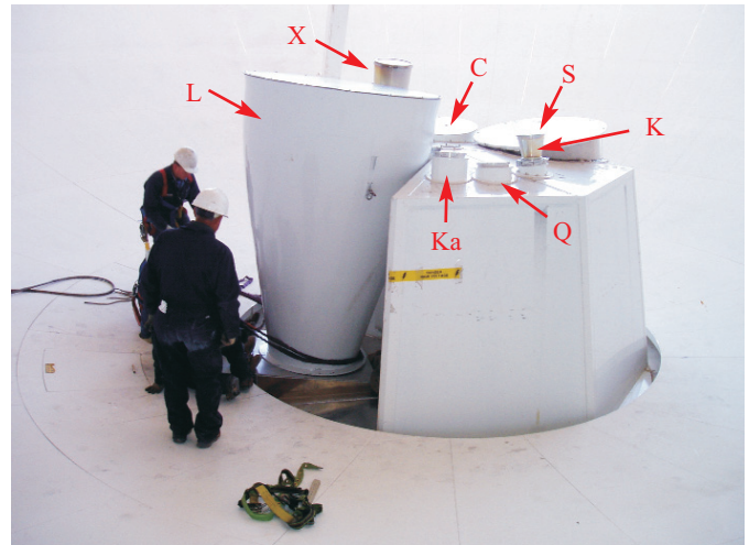
Figure 2. The EVLA cassegrain feeds, as labeled. The frequency ranges of each band are described in the receiver status portion of this article.
