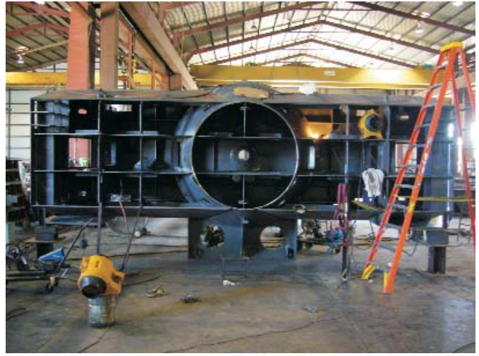
Figure 3. VertexRSI production antenna yoke base under construction in Texas, (August 23).
