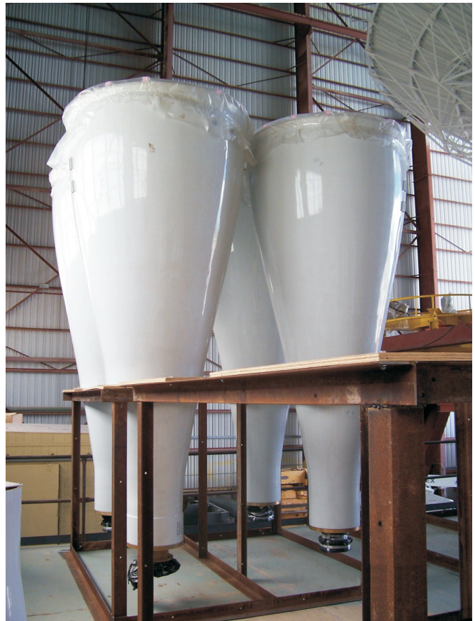
Figure 1. EVLA 1–2 GHz feed horns.
