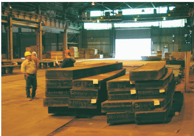
Azimuth Track Team member Dennis Egan (in yellow hard hat) inspecting the first set of the new GBT track base plates at Mittal Steel in Coatesville, PA..
