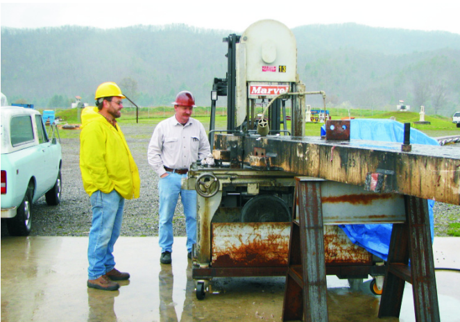
Figure 2. Modification of an original base plate to be used as a transition piece for driving the telescope onto the new track section. NRAO employees Mike Hedrick (left) and Harry Morton (right) are inspecting the piece.
