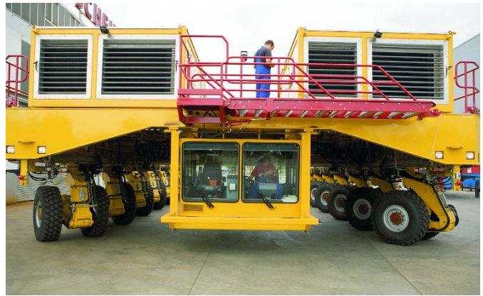
Figure 5. The first of two ALMA antenna transporters has been completed and has passed its initial operational tests.
