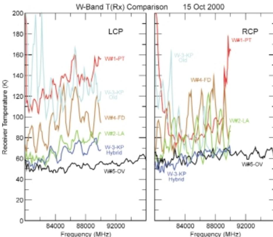
Laboratory measurements of receiver temperatures for the original four receivers, the hybrid system now at Kitt Peak, and the first new receiver.
