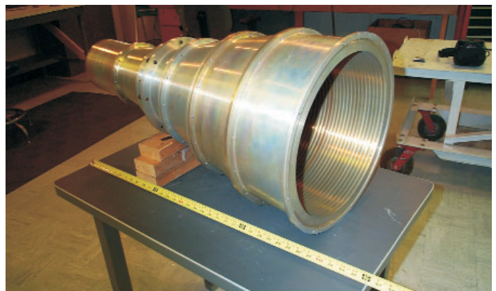
Figure 2. EVLA L-Band Feed Scaled Model, designed by CDL and machined in Green Bank.
