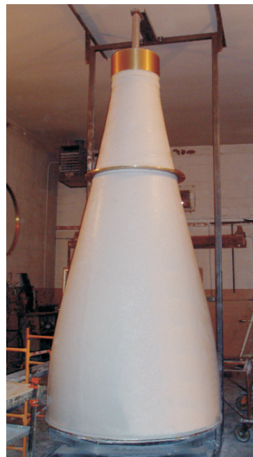
Completed L Band feed horn. Diameter 1.6 m, length 3.7 m.
