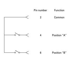
Figure 10. Indicator function diagram
