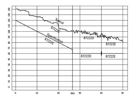
Figure 12. Agilent 87222C/D/E isolation versus frequency
