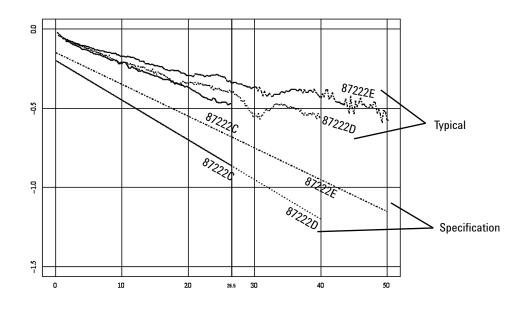
Figure 11. Agilent 87222C/D/E insertion loss versus frequency
