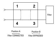
In the signal reverse configuration, a device can be connected across two diagonal ports of the 87222C/D/E transfer switch. This will allow the signal direction through the device to be reversed. See Figure 4.
