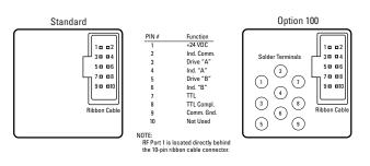
Figure 8. Drive connections
