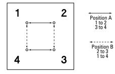
Figure 7. RF port connections
