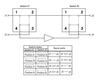
Figure 6. Bypassing an active device
