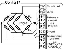
This is a combination of Config 1 for the reference channel and Config 3 for measurement channels.
