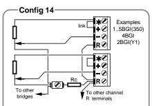
The bridge completion resistor is shared between channels. Its value is equal to the nominal value of the "unknown" resistor. The configuration is similar to Config 11 - no reference channel is needed.
