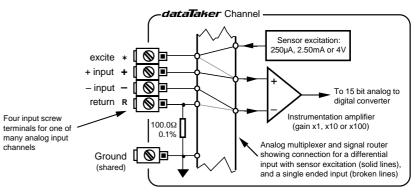
A Standard dataTaker Analog Input Channel
