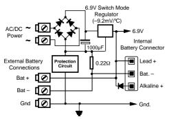
**Caution**: If a DC supply is grounded, it MUST be a negative ground. An AC supply MUST NOT be grounded.
