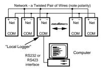
The computer can be connected to any dataTaker (referred to as the local logger) in the network through its RS232 COMMS port. Data is returned to the COMMS port of the local logger. P21 will allow this return address to be over ridden (see "Parameters" on page 11).
