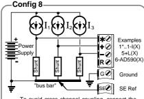
To avoid cross channel coupling, connect the bottom of the shunts with the minimum of shared resistance to the SE ref. take-off point.
