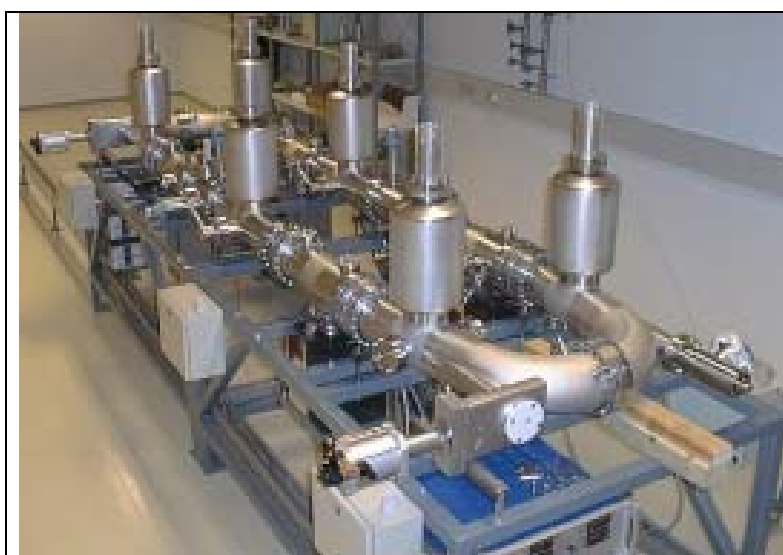
Figure 5a: Photograph of the ELISA electrostatic storage ring at the University of Aarhus. In addition, a double (merged) ESR ring system is in the final phases of construction at Stockholm University (Schmidt et al. 2008).
