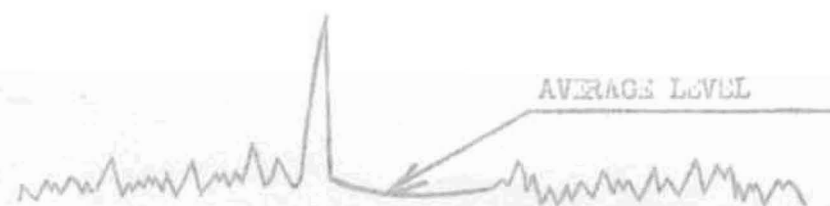
(c) WITH REJECTION CIRCUIT AND TRAILING EDGE ELIMINATOR FIG. 9 WAVEFORMS IN SCMA CIRCUITS
