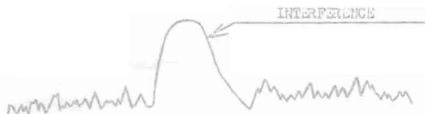
(a) RECEIVER OUTPUT WITH AN INTERFERING BURST
