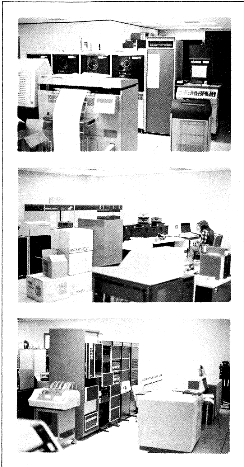
Figure 7-3. Photographs of some of the hardware of the off-line computer system in the computer room of the VLA control building: (a) DEC-10 tape drives, printer, card reader, and (on right) DISPLAY film recorder; (b) DEC-10 CPU, memory, and disks; and (c) part of SORTER/GRIDDER mapping system.
