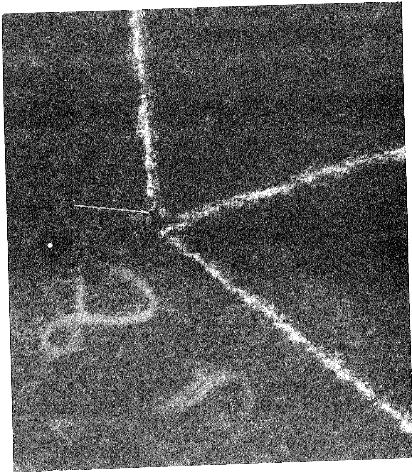
Figure 14. Enlargement of area of plate printed in Figure 14 showing target on stake (arrow). Actual diameter of target dot is 6mm; diameter of image on plate is 50 microns. Head of eight penny finishing nail in center of larger target lying on ground to left is clearly discernible on original plate.
