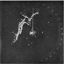
Fig. 63. A typical PPI picture. Normal, indirect, multiple and side echoes are showing.
