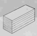
This is material with the grain of all the laminae running in the same direction. It is suitable for parts subject to tensile stresses or to bending, and is also highly resistant to torsion and to impact forces. It is easily machined and can readily be threaded or tapped.
