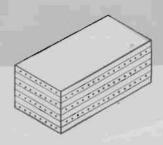
This is material with the grain of adjacent laminations at right angles. Its high compressive strength in the direction of its thickness, and rigidity, makes it very suitable for insulating blocks or panels.
