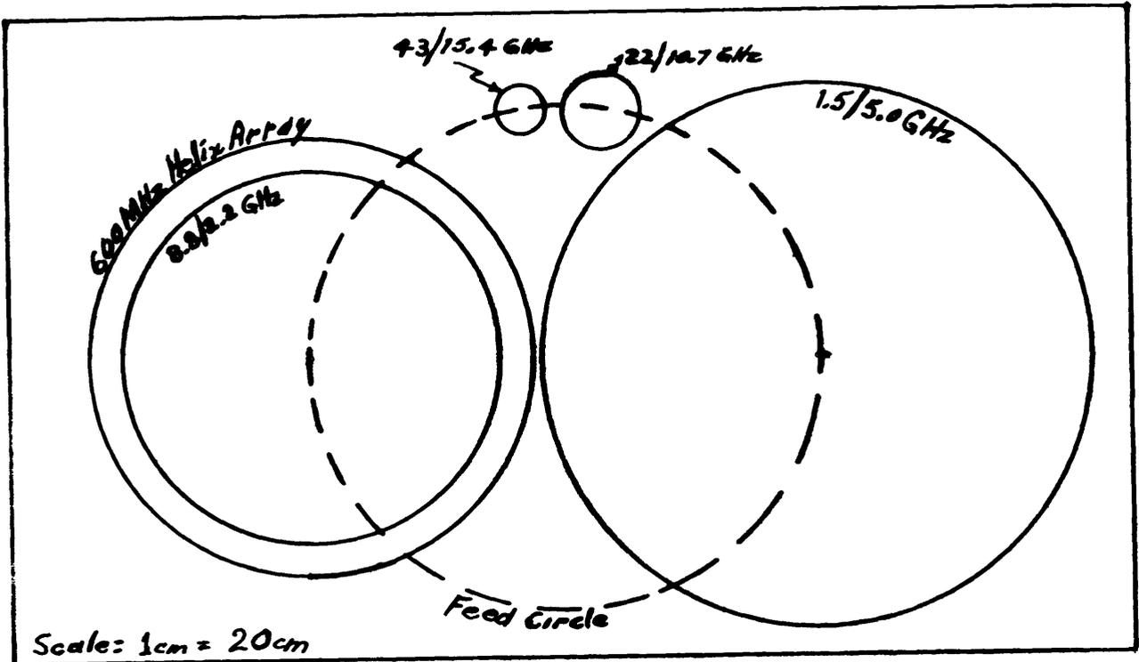
Figure III-8 Proposed Feed Layout
