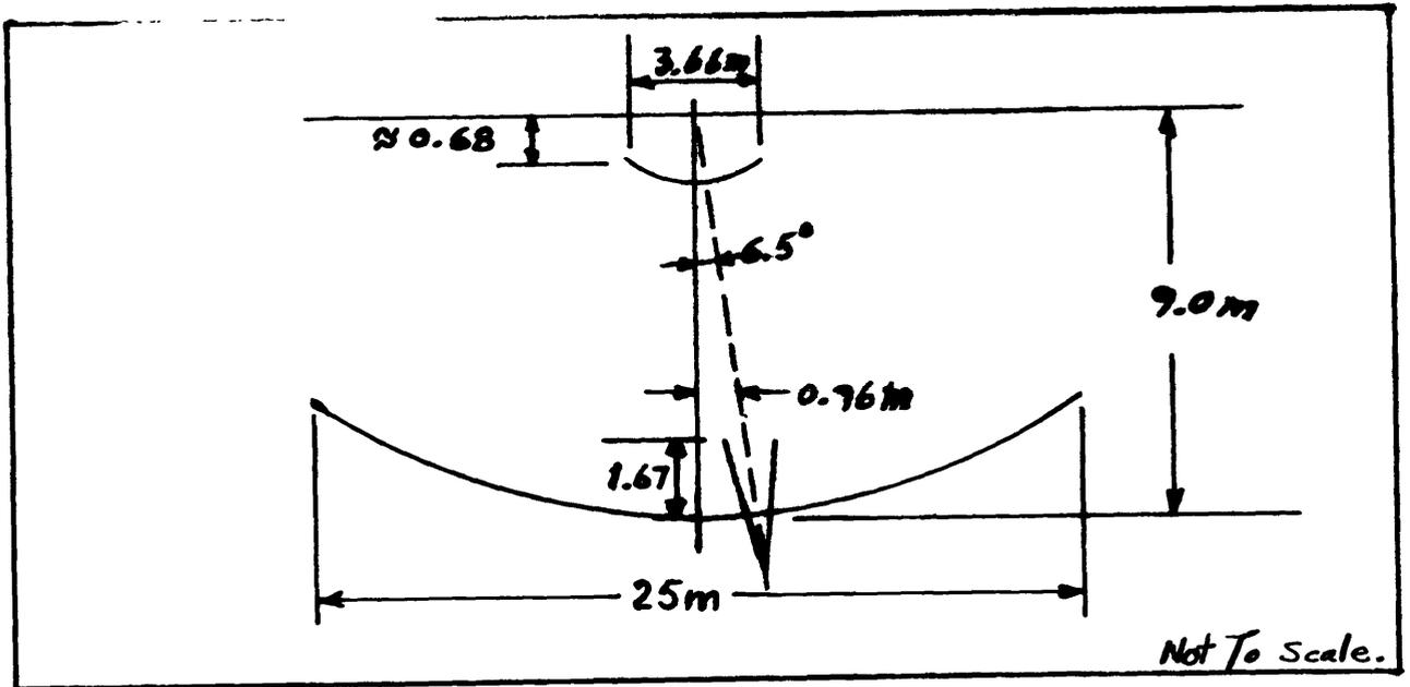
Figure III-7 Proposed Cassegrain Geometry
