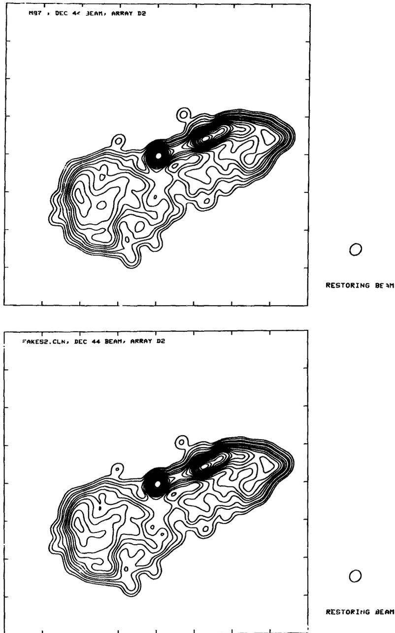
Figure III-5 a) A test source based on the 600 highest map cells in a VLA map of M87 which has been convolved with the CLEAN beam of Array D2 for observations at  $44^\circ$  declination. The test source is scaled down to a hypothetical size appropriate for VLBI observations. The contour levels are -1, -0.5, 0.5, 1, 2, 3, 5, 7, 9, 12, 15, 20, 25, 30, 35, 40, 50, 60, 70, and 80 percent of the peak.
