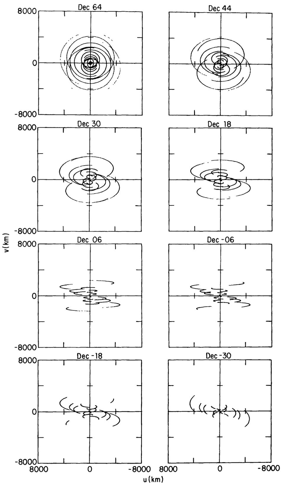
Figure III-3 Transfer functions for Array D2 showing only the baselines to the VLA. When the Array is used with the VLA, these baselines will have about five times the sensitivity of the others.
