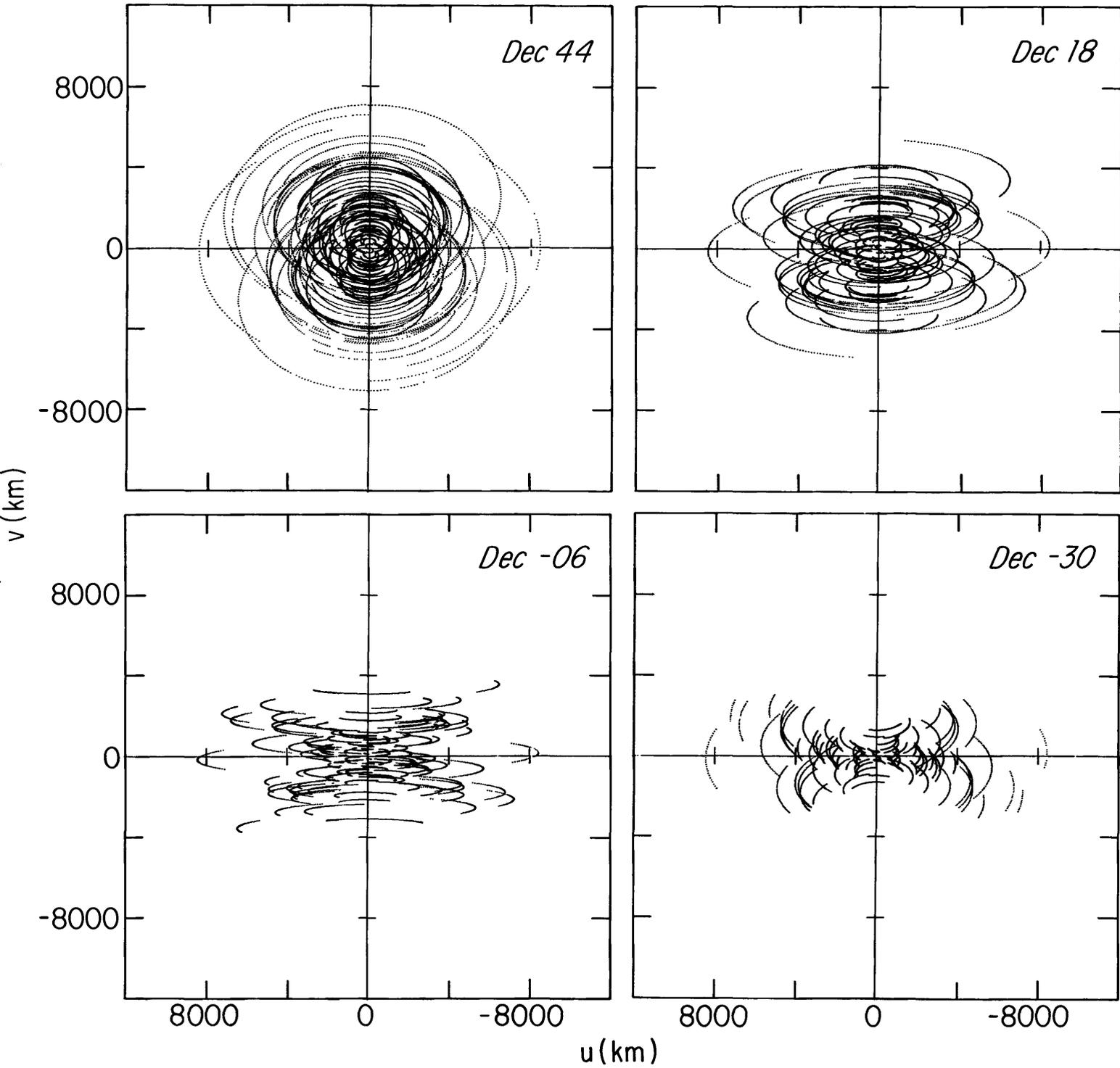
Figure III-6d The transfer functions for Array D2 plus Arecibo.
