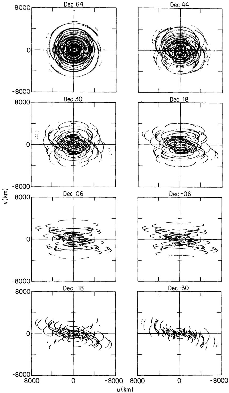
Figure III-2 Transfer functions for Array D2 at declinations centered in bands, each of which contains 10% of the sky.
