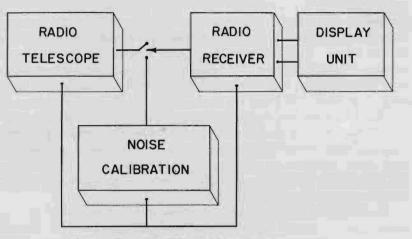
FIG. 1. The equipment used by radio astronomers.
