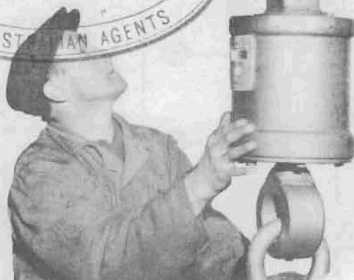
A type U PIAB dynamometer is used here for load checking a traverse.
